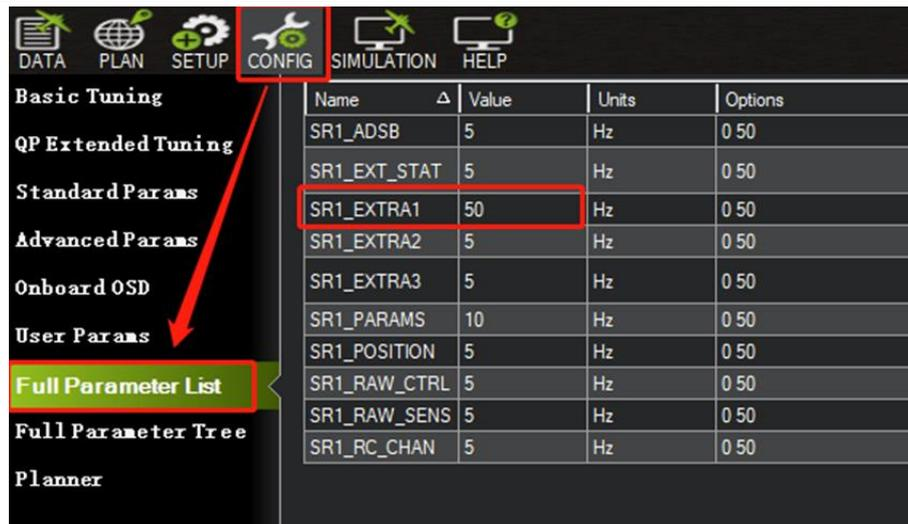
After configuration, it is necessary to “Write Parameters” and reboot the flight controller to take effect.
