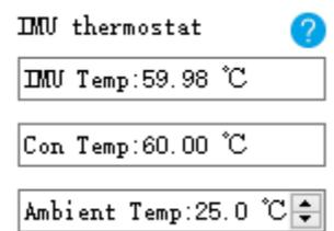
Before calibration, please input the environment temperature of your operating field, the software will start to calculate the target IMU constant temperature so that IMU can reach the temperature fast after powering on gimbal camera. The software is showing IMU temperature in real-time.
