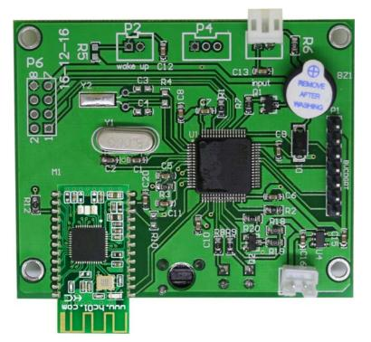
No copper can be applied and no wires can be routed under the antenna part of the module, otherwise the signal will be affected adversely. It is recommended that the bottom plate of the antenna may be hollowed out and the antenna be as close to the board as possible.
