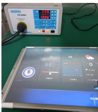
3.1 Electrostatic discharge test
