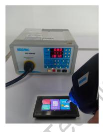
3.1 Electrostatic discharge test
